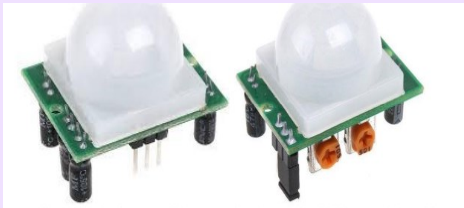
Figure.2 Motion detector module uses a motion detector IC and PCB mounted Fresnel lens
